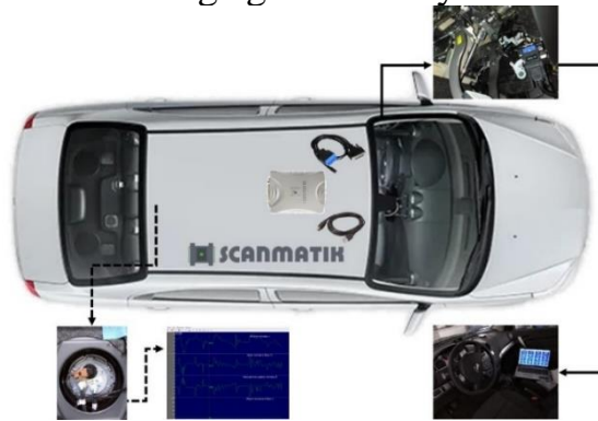
Fig.5. Recording the parameters of the vehicle in the driving mode through the scanmatic diagnostic device
