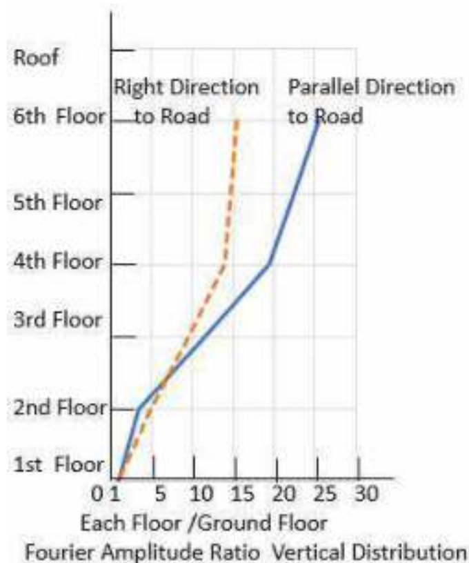
Fig.25 Vertical distribution of two horizontal vibrations.
