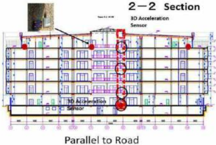
Fig.6. Sensor vertical location section elevation (along 2-2 line) of main building and accelerometer position in first, second, third measurement.
