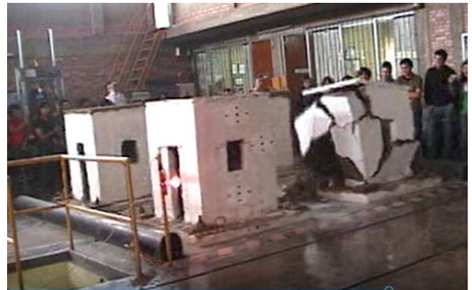
Fig.2 Educational Shaking Table Test in Peru Catolica Uni.
