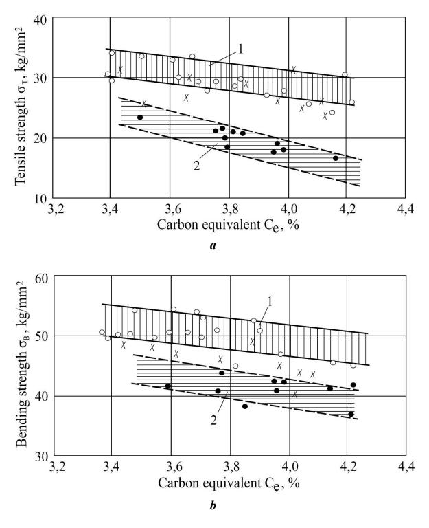
Figure 1. The effect of the carbon equivalent on  $\sigma_T$  (a) and  $\sigma_B$  (b) for gas (1), coke (2) cupolas, gas cupola with blank spike (x)
