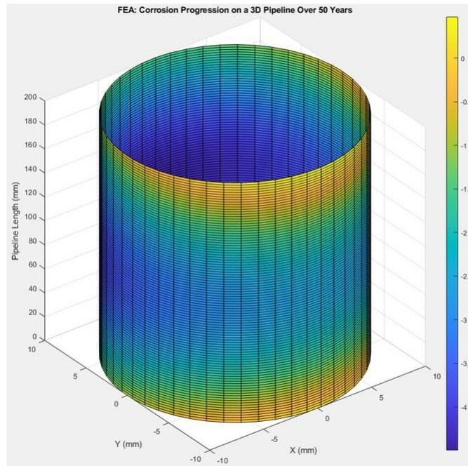
Fig. 1. FEA Simulation of Uniform Corrosion in a Metal Pipeline
