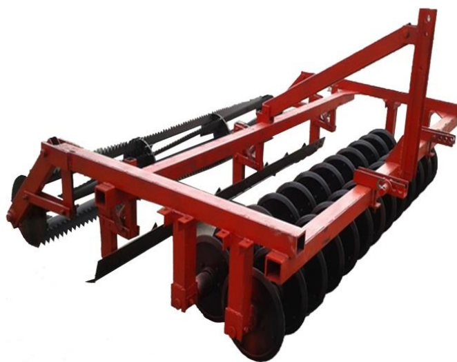
Figure 1. A combination machine used in the cultivation of newly plowed fields
