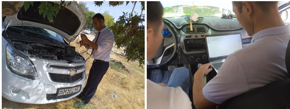
Figure 3. The process of connecting the computer to the engine gas electronic control unit and changing the petrol -gas mode indicators
